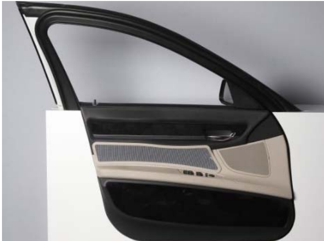
BMW Intelligent Thermal Management with Infrared Heating
